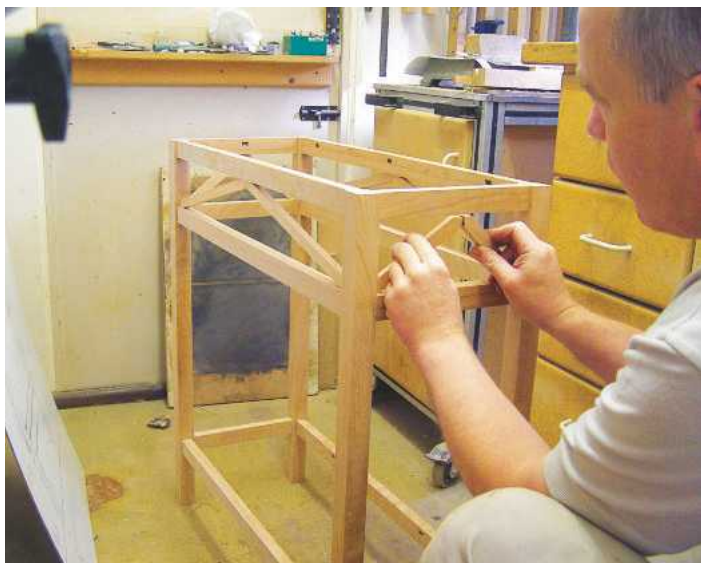
▲ Pic.11 The infill rails are inserted in pairs, and hold each other in place while the glue dries
